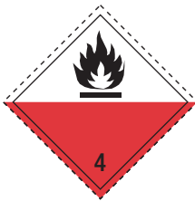
(No. 4.2) Class 4.2 Substances liable to spontaneous combustion Symbol (flame): black. Background: upper half white, lower half red. Figure '4' in bottom corner.
