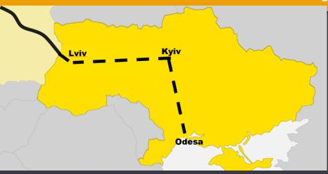
~896-990 km of Odessa-Kyiv-Lviv (EU border) will provide a high speed connection for 6 UA regions with total passenger traffic on these routes of 137 mln in 2017. Passenger train speed about 250 km/h.
